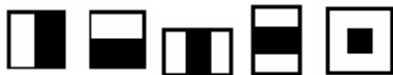
Figure 2. The basic Haar-like features which were used by Viola and Jones [2001] in their frontal face detector.
