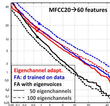
Figure 3: The effect of number of eigenchannels for JFA with  $\mathbf{D}$  trained on data and full JFA. Results on NIST 2006 data.
