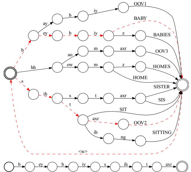
Figure 3: Toy example of lexical FST  $L$  containing all recognized OOVs and IVs and a given sub-word sequence, represented below as input FST  $I$ . The composition  $I \circ L$  is dashed.
