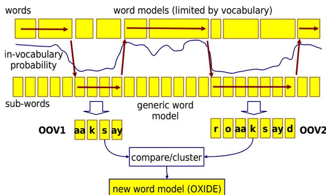
Figure 1: OOV recognition with hybrid word/sub-word model and comparison of sub-word sequences, extracted from one-best recognition output.
