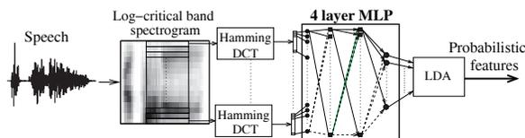
Fig. 2. Block diagram of Probabilistic feature extraction
