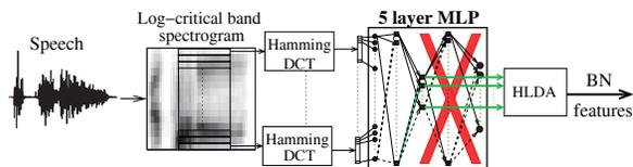
Fig. 1. Block diagram of Bottle-Neck feature extraction
