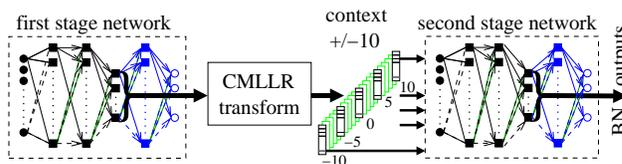
**Fig. 1.** Stacked Bottle-Neck Neural Network feature extraction.
