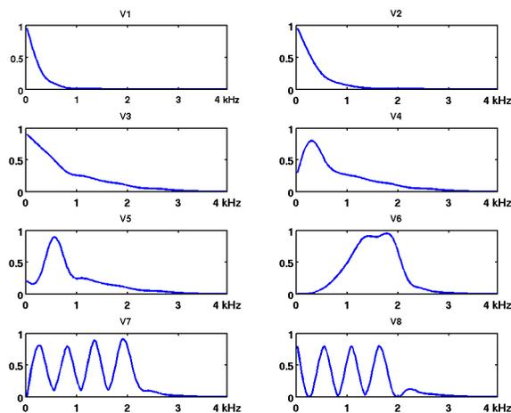
Fig. 3. Frequency characteristics of noise filters.
