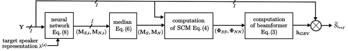
Figure 1: The entire processing with multichannel signal  $\mathbf{Y}_i$  as input and estimate of the target speaker signal  $\tilde{S}_{i_{\text{ref}}}$  as the output.
