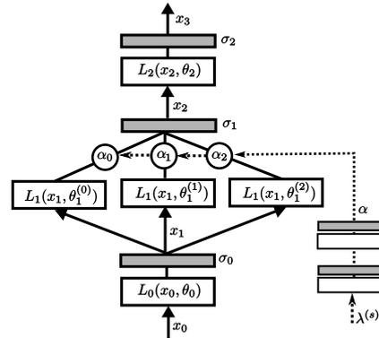
Figure 3: Scheme of speaker adaptive layer configuration.
