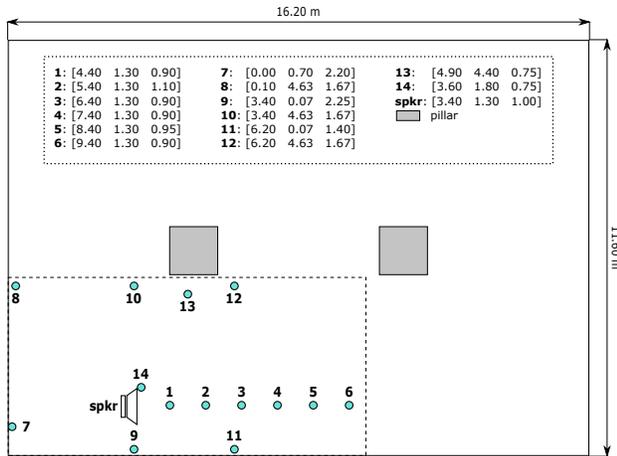
**Fig. 1.** Floor plan of the room in which the retransmission took place. Coordinates are in meters and lower left corner is the origin. Dashed rectangle borders area displayed in Figure 3.
