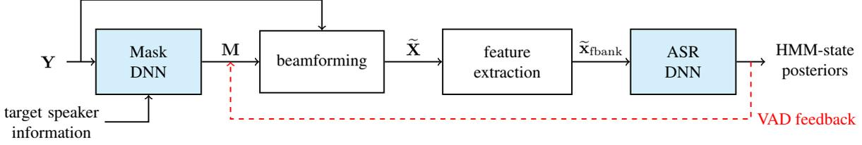
**Fig. 2.** The processing chain with the multichannel signal  $\mathbf{Y}$  as input and the estimated HMM-state posteriors as the output. The trainable blocks are shown in blue. The red dashed line shows the VAD feedback as described in Section 3.2.
