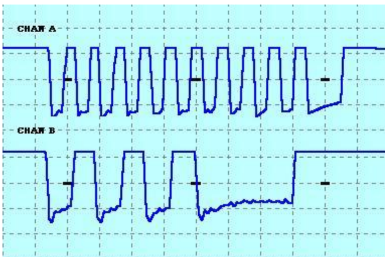
Figure 3: Scan code for the "Q" key (15h) being sent from a keyboard to the computer. Channel A is the Clock signal; channel B is the Data signal.
