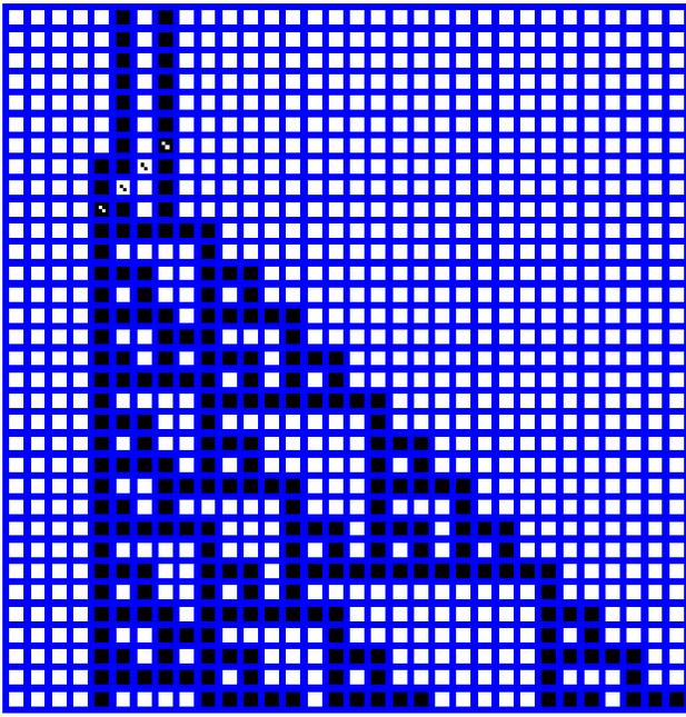
Fig. 10. Emergent behavior of the CA controlled by the transition function from Figure 9. The result of the product  $3 \times 3 = 9$  is shown within the cells marked by two dots in the upper-left part of the CA. The diagonal cell setup was considered according to Figure 3c.
