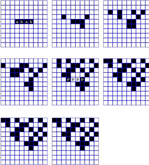
Fig. 4. Example of an evolved CA development performing the multiplication  $3 \times 3 = 9$ . White cell in the CA represents the state 0, black cell represents the state 1. The input operands as well as the resulting product are considered in direct binary representation using the cell states (the operands  $a = b = (11)_{bin} = (3)_{dec}$ , the product  $p = (1001)_{bin} = (9)_{dec}$ ). Both the operand bits and product bits are interpreted from MSB to LSB as from left to right.
