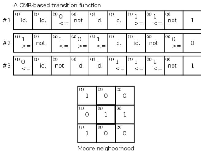
Fig. 2. Example of a transition function represented by conditionally matching rules. Note that the identity function ( $id$ ) and negation ( $not$ ) do not need any state value in the conditional part of the CMR because the decision of matching their part of CMR is based only on evaluating the appropriate cell state in the cellular neighborhood. The thick rectangle denotes the cell for which the new state ought to be calculated.
