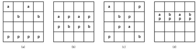
Fig. 3. The setups for input and output cell arrangements in cellular automata: (a) separated, (b) alternating, (c) diagonal, (d) shared. In each of the setups,  $a$  and  $b$  denote the input cells whose states represent values for the 2-bit operands,  $p$  denote the output cells in which the resulting product is expected after the CA development. Note that in the shared setup (d) the result is expected in the same cells as the input operands.
