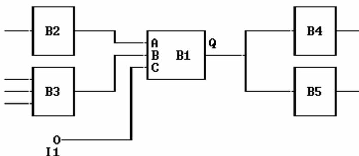
We will show program in Linda language which describes the B1 block. This block has three inputs A, B, C and one output Q. Value of the Q output is dependent on the input values and the model-time. We will show both the continuous simulation approach and the synchronous demand-driven simulation approach.
