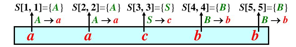
**GP Based on CNF:** Example 2/5 G = (N, T, P, S), where  $N = \{A, B, C, S\}, T = \{a, b\}, P = \{S \rightarrow AC, C \rightarrow SB, A \rightarrow a, B \rightarrow b, S \rightarrow c\}$ **Question:**  $aacbb \in L(G)$ ?
