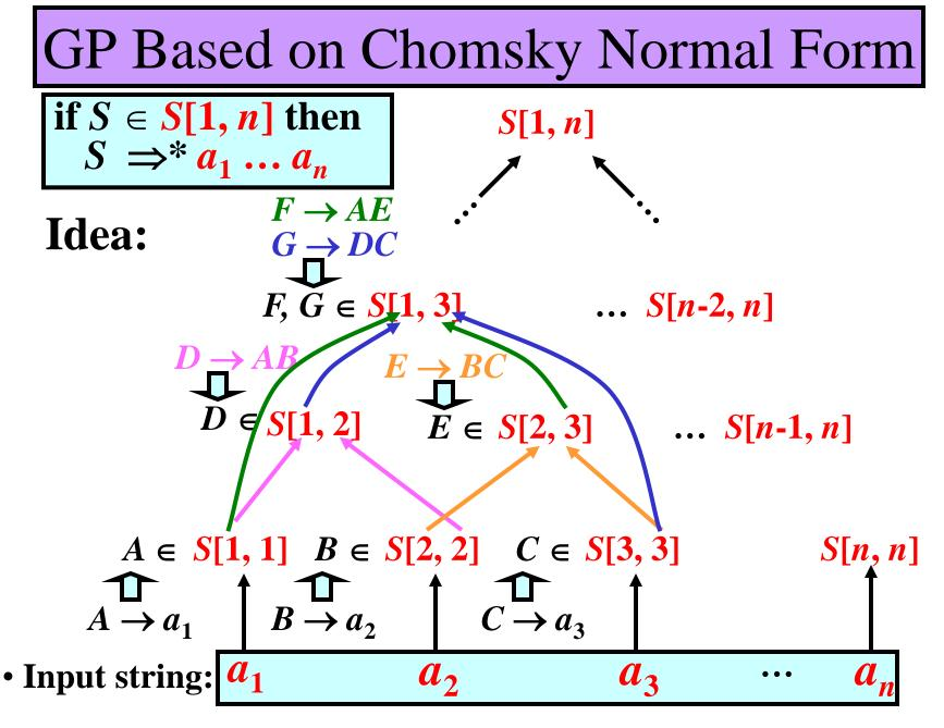
Algorithm: GP Based on CNF • Input: G = (N, T, P, S) in CNF,  $w = a_1...a_n$ • Output: YES if  $w \in L(G)$ NO if  $w \notin L(G)$
