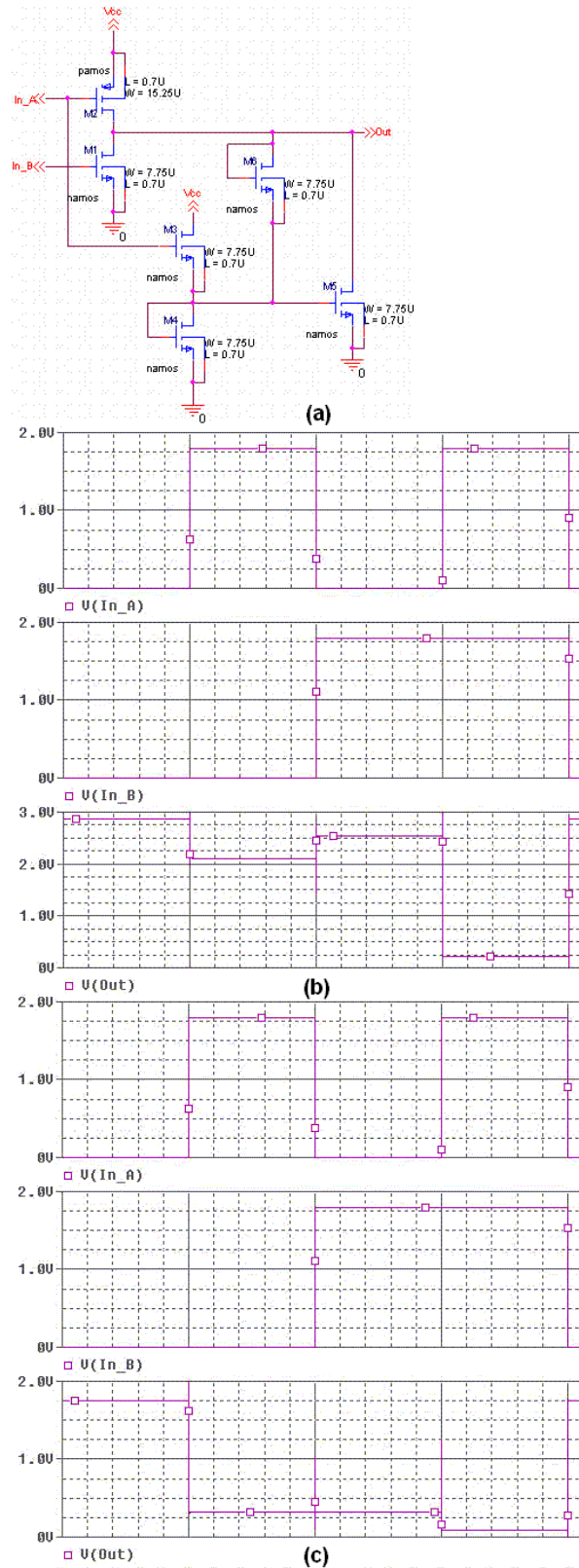
Figure 1. (a) NAND/NOR gate taken from [8], (b) NAND when V_{dd} = 3.3V , (c) NOR when V_{dd} = 1.8V
