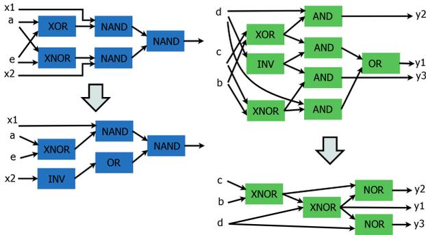
Fig. 4. Example 1-3: Subcircuits of  $G$  optimized by CGP.
