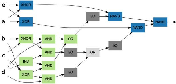
Fig. 3. Example 1-2: Decomposition of  $G$  according to Alg. 2.
