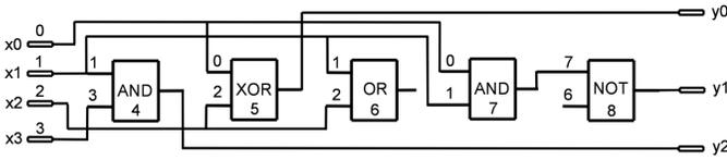
Fig. 1. A candidate circuit represented by CGP with parameters:  $n_i = 4$ ,  $n_o = 3$ ,  $n_c = 5$ ,  $n_r = 1$ ,  $l = 4$ ,  $\Gamma = \{0^{AND}, 1^{OR}, 2^{XOR}, 3^{NOT}\}$ . Chromosome: 1, 3, 0; 0, 2, 2; 1, 2, 1; 0, 1, 0; 7, 6, 3; 5, 8, 4.
