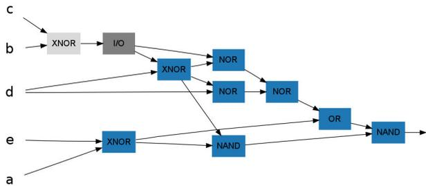
Fig. 5. Example 1-4: Optimized subcircuits are merged and another decomposition is applied.
