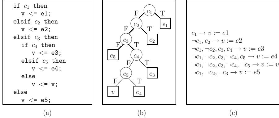
**Fig. 4.** Synthesis of behavioural rules wrt. the conditions passed till a certain assignment can be fired: (a) a normalized VHDL `if` statement, (b) the tree representing branching conditions, (c) the set of behavioural rules for variable  $v$
