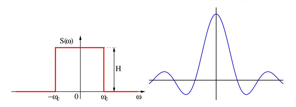
$$x(t) = \frac{1}{2\pi} \int_{-\infty}^{\infty} X(j\omega) e^{+j\omega t} d\omega = \frac{1}{2\pi} \int_{-\omega_c}^{\omega_c} H e^{+j\omega t} d\omega = \frac{H}{2\pi} \int_{-\omega_c}^{\omega_c} e^{+j\omega t} d\omega = \frac{H}{2\pi} 2\omega_c \operatorname{sinc}(\omega_c t) = \frac{H\omega_c}{\pi} \operatorname{sinc}(\omega_c t)$$
