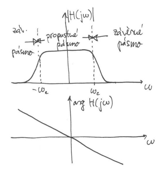
Transfer of a signal through a system with  $H(j\omega)$
