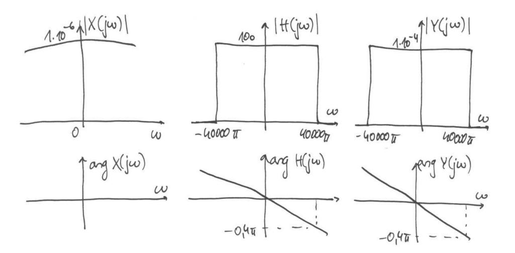
The result is a square signal with linear phase. As the last step, an inverse Fourier transform has to be applied.
