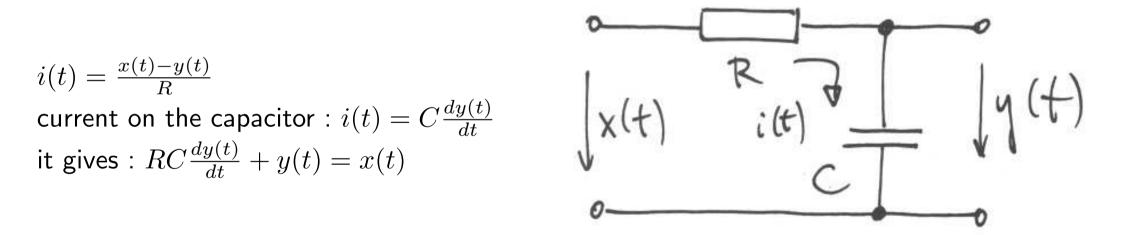
$\tau = RC$  is so called **time constant** of the system. The coefficients of the differential equation are :  $a_1 = \tau$ ,  $a_0 = 1$ ,  $b_0 = 1$ .
