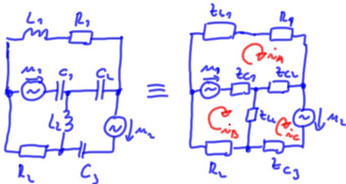
$$\dot{i}_A : (t_{L1} + t_{L2}) I_A + t_{C2} (I_A - \frac{I_B}{t_{C1}}) + t_{C1} (I_A - I_B) - U_A = 0$$
