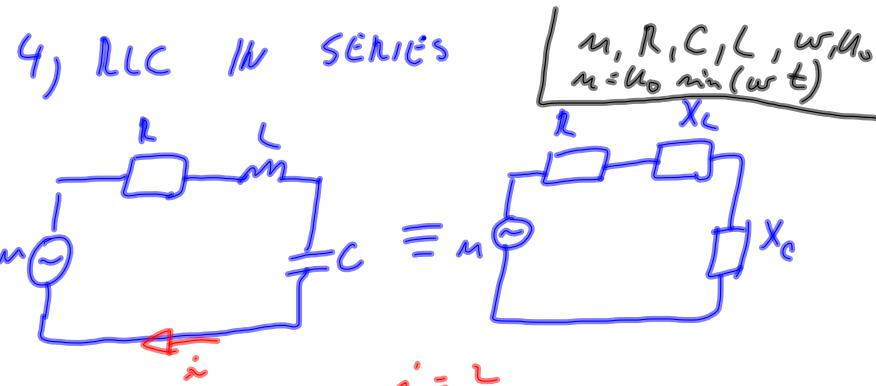
$$\begin{aligned} i &= \frac{u}{Z_{EQV}} \\ i &= I_0 \sin(\omega t + \varphi) \end{aligned}$$
