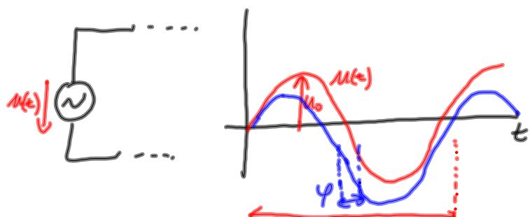
$$U(t) = U_0 \sin(\omega t + \varphi) \quad \text{PHASE SHIFT}$$
