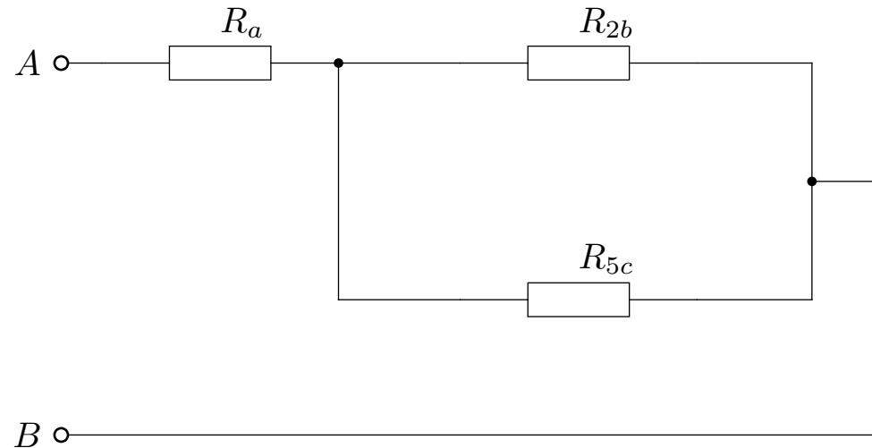
$$R_{2b} = R_b + R_2 = 37,5 + 200 = 237,5\Omega$$
