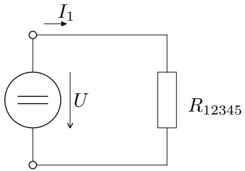
$$R_{12345} = R_1 + R_{2345} = 3000 + 3250 = 6,25k\Omega$$
