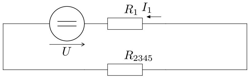
$$R_{2345} = \frac{R_{234} \cdot R_5}{R_{234} + R_5} = \frac{38 \cdot 20}{38 + 20} = 13,1\Omega$$
