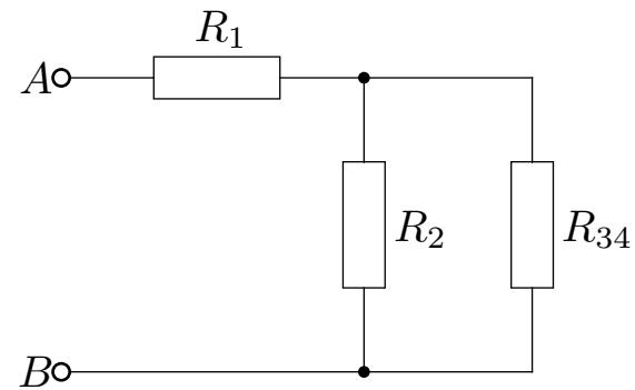
$$R_{34} = R_3 + R_4 = 200\Omega + 200\Omega = 400\Omega$$
