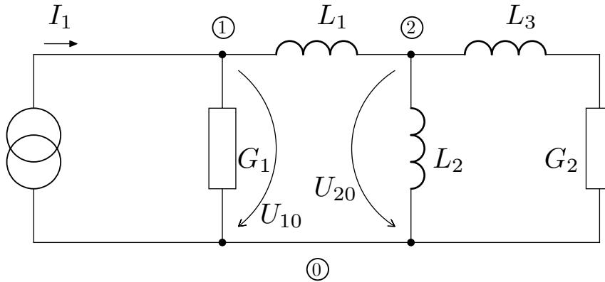
$$\begin{pmatrix} G_1 + \frac{1}{j\omega L_1} & -\frac{1}{j\omega L_1} \\ -\frac{1}{j\omega L_1} & \frac{1}{j\omega L_1} + \frac{1}{j\omega L_2} + Z_{L3G2} \end{pmatrix} \cdot \begin{pmatrix} \hat{U}_{10} \\ \hat{U}_{20} \end{pmatrix} = \begin{pmatrix} \hat{I}_1 \\ 0 \end{pmatrix}$$
