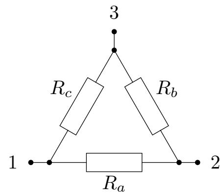
$$R_a = R_{10} + R_{20} + R_{10} \cdot \frac{R_{20}}{R_{30}}$$
