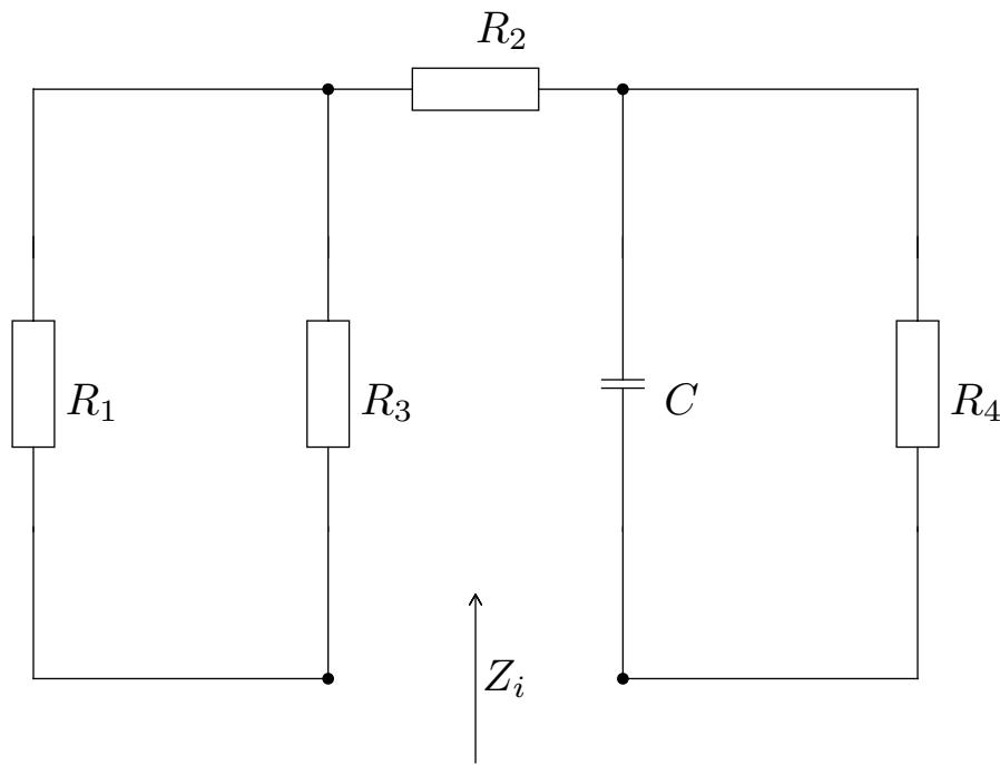
$$\hat{Z}_i = \frac{R_1 \cdot R_3}{R_1 + R_3} + R_2 + \frac{-R_4 \cdot \frac{j}{\omega C}}{R_4 - \frac{j}{\omega C}} = \frac{200 \cdot 120}{320} + 160 - \frac{80 \cdot 60j}{80 - 60j} = (263, 8 - 38, 4j)\Omega$$
