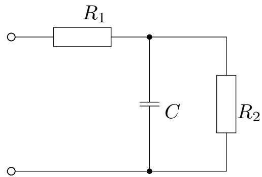
$$\begin{aligned}R_1 &= 800\Omega \\R_2 &= 200\Omega \\C &= 5nF\end{aligned}$$
