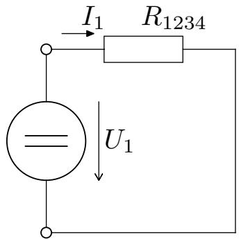
$$R_{1234} = R_1 + R_{234} = 20 + 50 = 70\Omega$$
