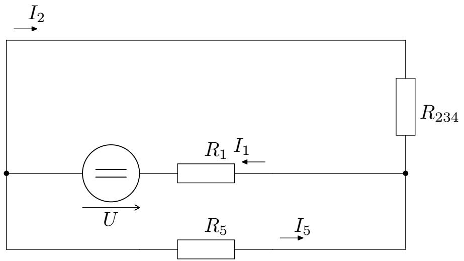
$$R_{234} = R_2 + R_{34} = 30 + 8 = 38\Omega$$
