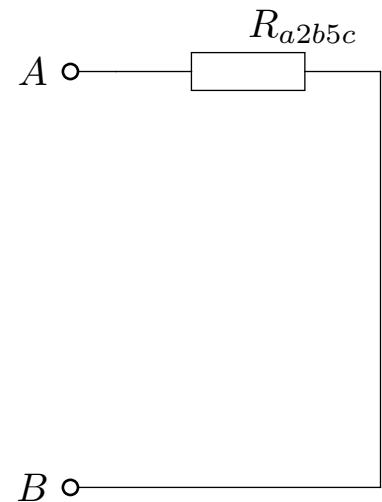
$$R_{a2b5c} = R_a + R_{2b5c} = 50 + 173,94 = 223,94\Omega$$
