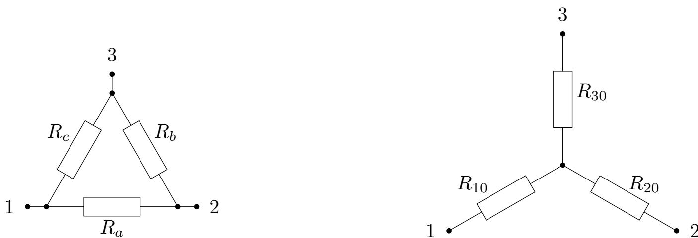
$$R_{10} = \frac{R_a \cdot R_c}{R_a + R_b + R_c}$$
