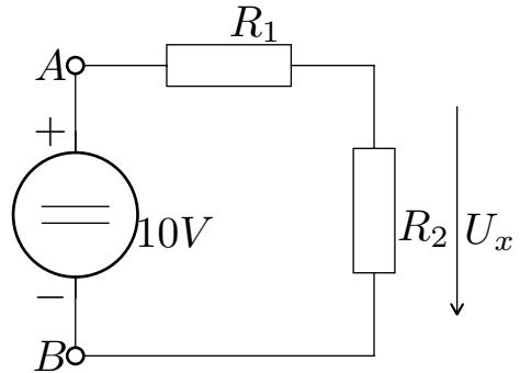
$$R_{12} = R_1 + R_2 = 200 + 200 = 400\Omega$$
