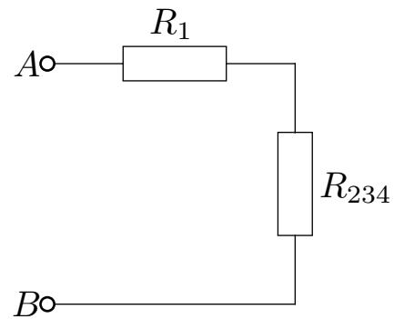
$$R_{234} = \frac{R_2 \cdot R_{34}}{R_2 + R_{34}} = \frac{400\Omega \cdot 400\Omega}{400\Omega + 400\Omega} = 200\Omega$$
