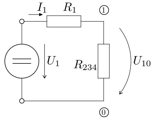
$$R_{234} = \frac{R_2 \cdot R_{34}}{R_2 + R_{34}} = \frac{100 \cdot 100}{100 + 100} = 50\Omega$$
