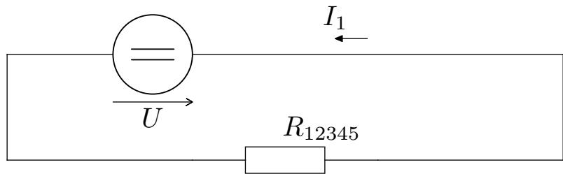
$$R_{12345} = R_1 + R_{2345} = 2 + 13,1 = 15,1\Omega$$
