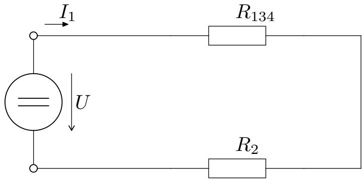
$$R_{134} = \frac{R_3 \cdot R_{14}}{R_3 + R_{14}} = \frac{3000 \cdot 5000}{3000 + 5000} = 1,875 k\Omega$$
