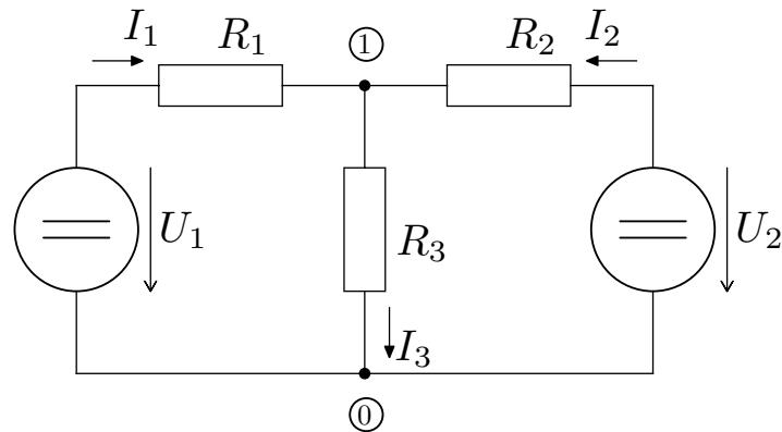
$$R_{23} = \frac{R_2 \cdot R_3}{R_2 + R_3} = \frac{20 \cdot 15}{20 + 15} = 8,571\Omega$$
