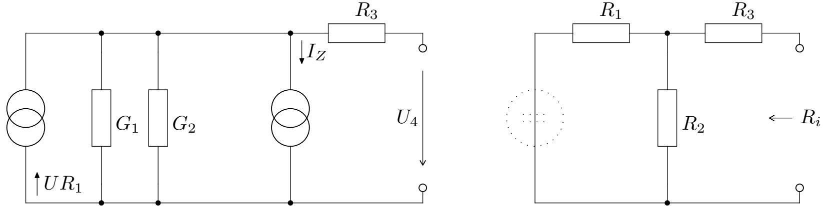
$$(G_1 + G_2)U_i = \frac{U}{R_1} \Rightarrow U_i = \frac{UG_1 - I_Z}{G_1 + G_2} = -6,6V$$
