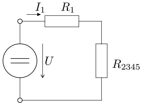
$$R_{2345} = \frac{R_2 \cdot R_{345}}{R_2 + R_{345}} = \frac{13000 \cdot 4333}{13000 + 4333} = 3,25k\Omega$$
