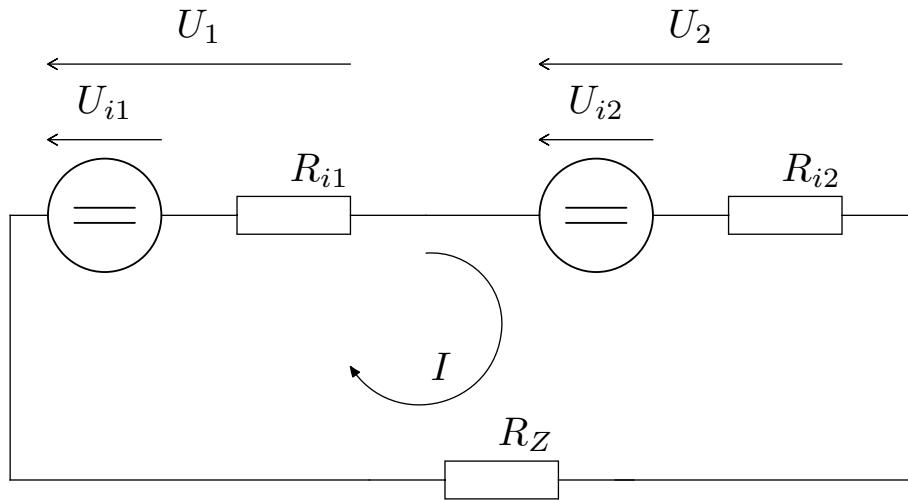
$$I_b = \frac{U_{i1} + U_{i2}}{R_{i1} + R_{i2} + R_Z} = \frac{1,6 + 1,2}{0,8 + 4 + 3} = 0,359A$$
