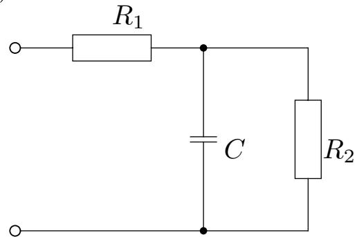
$$\hat{Z} = R_1 + \frac{R_2 \cdot \frac{1}{j\omega \cdot C}}{R_2 + \frac{1}{j\omega \cdot C}}$$
