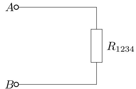
$$R_{1234} = R_1 + R_{234} = 100\Omega + 200\Omega = 300\Omega$$
