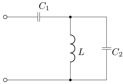
$$\hat{Z} = \frac{1}{j\omega \cdot C_1} + \frac{j\omega \cdot L \cdot \frac{1}{j\omega \cdot C_2}}{j\omega \cdot L + \frac{1}{j\omega \cdot C_2}}$$
