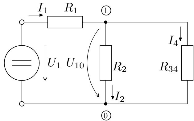
$$R_{34} = R_3 + R_4 = 50 + 50 = 100\Omega$$
