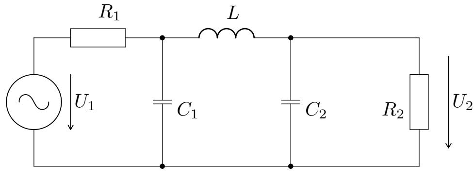
$$\begin{aligned}\hat{U}_1 &= 10V \\ f &= 100Hz \\ R_1 &= 200\Omega \\ R_2 &= 50\Omega \\ L &= 5H \\ C_1 &= C_2 = 50\mu F\end{aligned}$$
