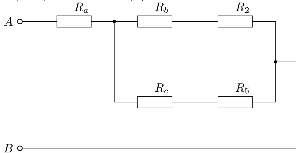
$$R_a = \frac{R_1 \cdot R_4}{R_1 + R_3 + R_4} = \frac{100 \cdot 400}{100 + 300 + 400} = 50\Omega$$
