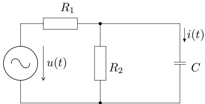
$$\begin{aligned} u(t) &= U_m \cdot \sin(\omega t) = 12 \cdot \sin(2 \cdot \pi \cdot 50 \cdot t) \\ R_1 &= 1k\Omega \\ R_2 &= 4k\Omega \\ C &= 10\mu F \end{aligned}$$
