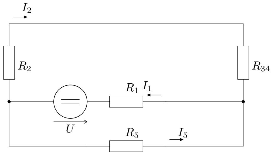
$$R_{34} = \frac{R_3 \cdot R_4}{R_3 + R_4} = \frac{40 \cdot 10}{40 + 10} = 8\Omega$$
