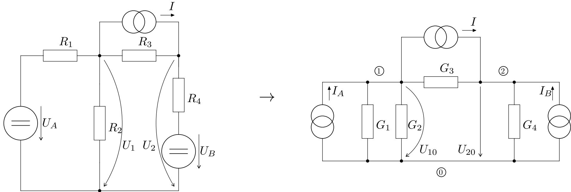
$$I_A = \frac{U_A}{R_1} = \frac{20}{20} = 1A \quad I_B = \frac{U_B}{R_4} = \frac{15}{40} = 0,375A$$
