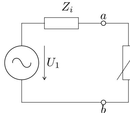
$$\hat{U}_1 = U_{1ef} \angle \alpha = \frac{33}{12} \angle 18^\circ = 23,33 \angle 18^\circ$$
