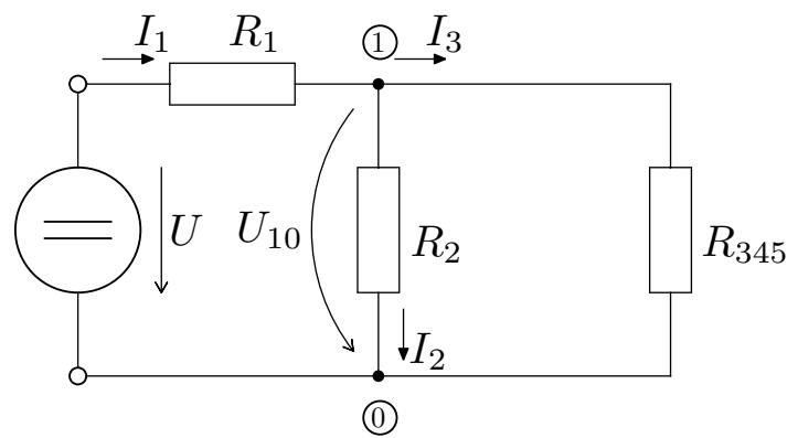
$$R_{345} = R_3 + R_{45} = 3000 + 1333,3 = 4,333 k\Omega$$
