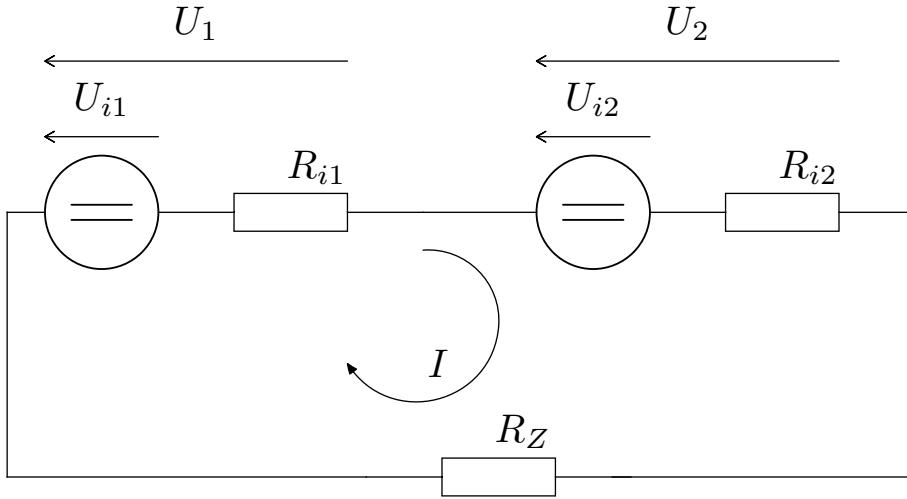
$$I_a = \frac{U_{i1} + U_{i2}}{R_{i1} + R_{i2} + R_Z} = \frac{1,6 + 1,2}{0,8 + 4 + 5} = 0,2857A$$
