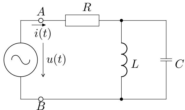
$$\begin{aligned} u(t) &= U_m \sin(\omega t + \varphi_m), U_m = 314V \\ \varphi_m &= 0, f = 50Hz \\ R &= 100\Omega \\ C &= 20\mu F \\ L &= 0,2H \end{aligned}$$
