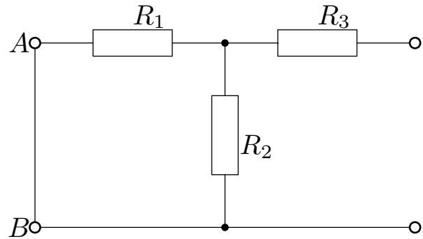
$$R_{12} = \frac{R_1 \cdot R_2}{R_1 + R_2} = \frac{200 \cdot 200}{200 + 200} = 100\Omega$$
