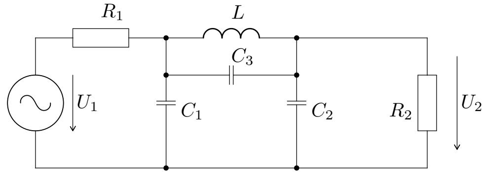
$$\begin{aligned}\hat{U}_1 &= 10V \\ f &= 100Hz \\ R_1 &= 200\Omega \\ R_2 &= 50\Omega \\ L &= 1H \\ C_1 &= C_2 = 50\mu F \\ C_3 &= 2,5\mu F\end{aligned}$$
