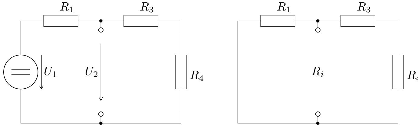
$$U_i = U \frac{R_3 + R_4}{R_1 + R_3 + R_4} = 20 \cdot \frac{10 + 40}{10 + 10 + 40} = 16, \overline{6}V$$
