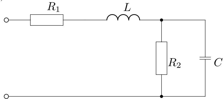
$$\begin{aligned}R_1 &= 10\Omega \\R_2 &= 50k\Omega \\L &= 180\mu H \\C &= 500pF\end{aligned}$$
