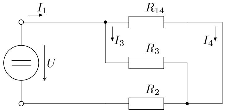
$$R_{14} = R_1 + R_4 = 3000 + 2000 = 5k\Omega$$
