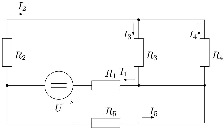
$$U_{R3} = U - R_1 I_1 - R_2 I_2 = 48 - 2 \cdot 3,178 - 30 \cdot 1,096 = 8,764 \text{ V}$$
