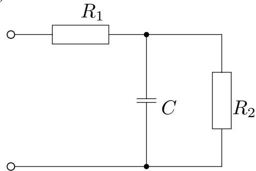
$$\hat{Z} = R_1 + \frac{R_2 \cdot \frac{1}{j\omega C}}{R_2 + \frac{1}{j\omega C}}$$
