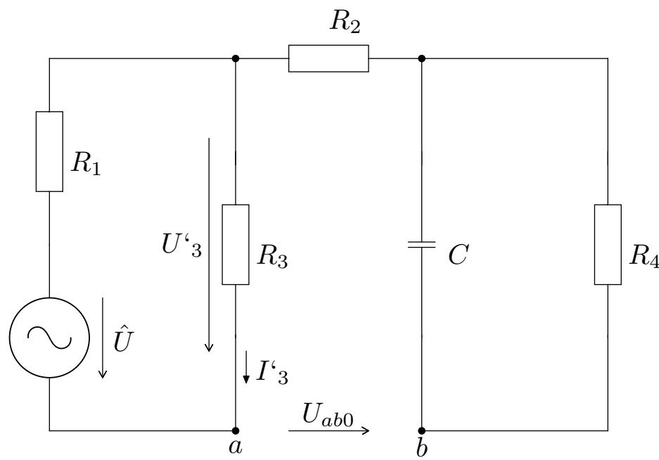
$$\begin{aligned}\hat{I}_3 &= \frac{\hat{U}}{R_1 + R_2} = \frac{40}{200 + 120} = \\ &= 0,125A\end{aligned}$$
