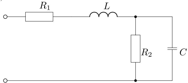
$$\hat{Z} = R_1 + j\omega \cdot L + \frac{R_2 \cdot \frac{1}{j\omega \cdot C}}{R_2 + \frac{1}{j\omega \cdot C}}$$
