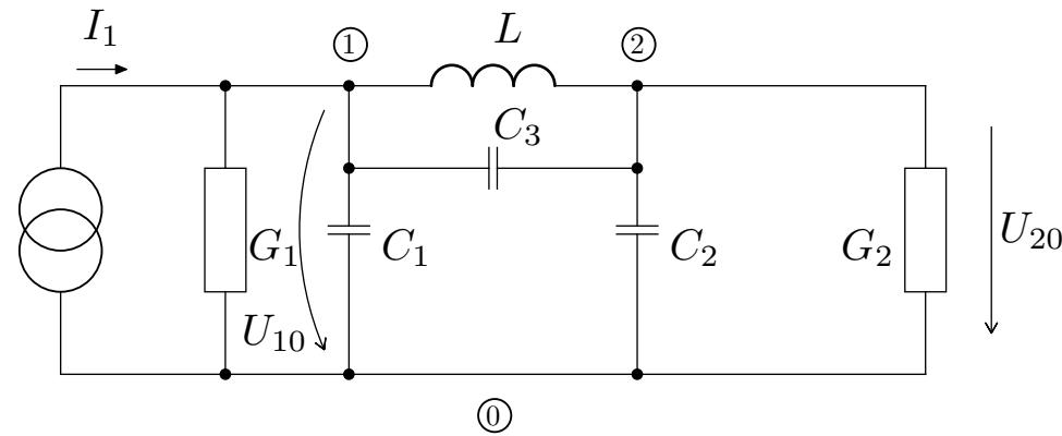
$$\begin{pmatrix} G_1 + j\omega C_1 + j\omega C_3 + \frac{1}{j\omega L} & -j\omega C_3 - \frac{1}{j\omega L} \\ -j\omega C_3 - \frac{1}{j\omega L} & G_2 + j\omega C_2 + j\omega C_3 + \frac{1}{j\omega L} \end{pmatrix} \cdot \begin{pmatrix} \hat{U}_{10} \\ \hat{U}_{20} \end{pmatrix} = \begin{pmatrix} \hat{I}_1 \\ 0 \end{pmatrix}$$
