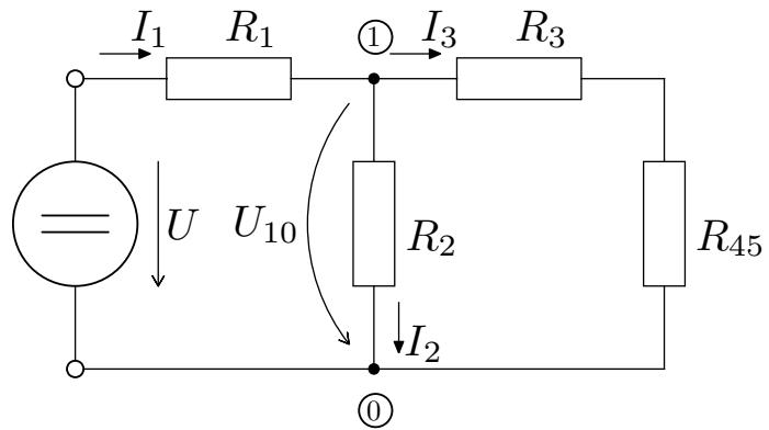
$$R_{45} = \frac{R_4 \cdot R_5}{R_4 + R_5} = \frac{2000 \cdot 4000}{2000 + 4000} = 1,3333k\Omega$$
