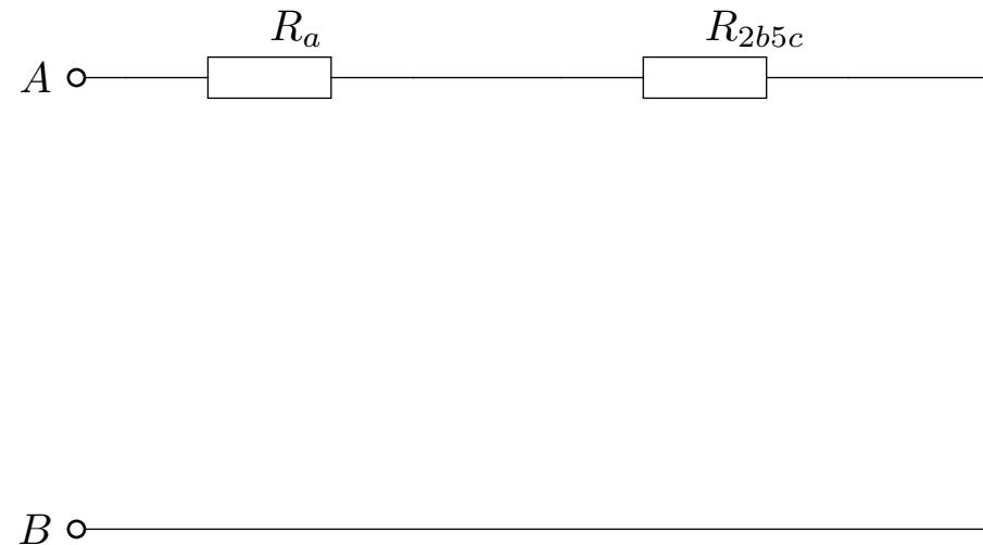
$$R_{2b5c} = \frac{R_{2b} \cdot R_{5c}}{R_{2b} + R_{5c}} = \frac{237,5 \cdot 650}{237,5 + 650} = 173,94\Omega$$
