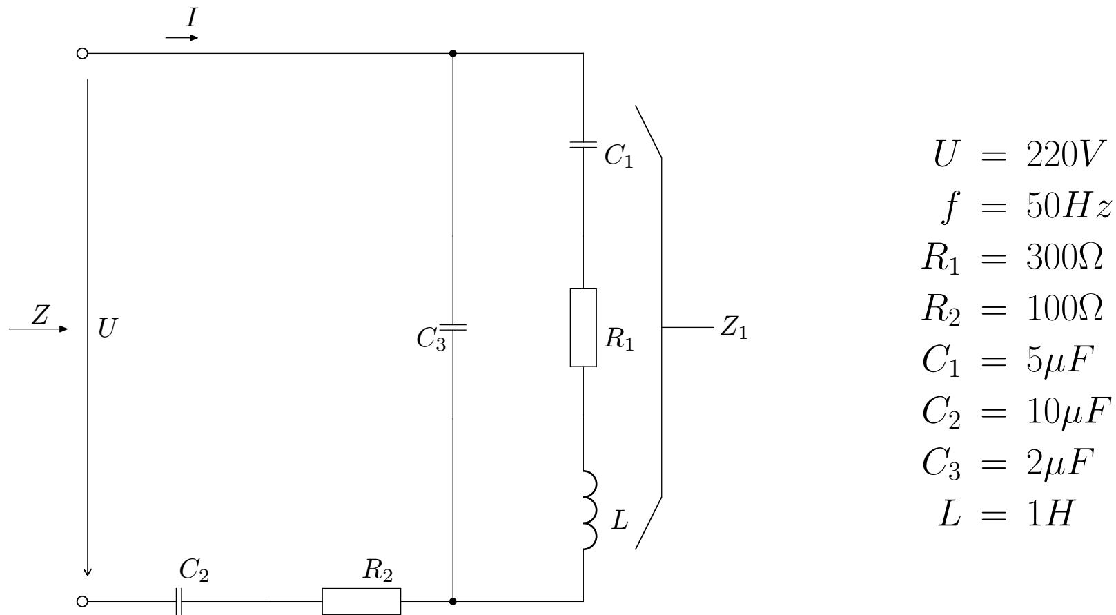
$$\begin{aligned}\hat{Z}_1 &= R_1 + j\omega L + \frac{1}{j\omega C_1} = 300 + j(2\pi \cdot 50 \cdot 1 - \frac{1}{2\pi \cdot 50 \cdot 5 \cdot 10^{-6}}) = \\ &= (300 - 322, 46j)\Omega = 440, 43\angle - 47, 07^\circ \Omega\end{aligned}$$
