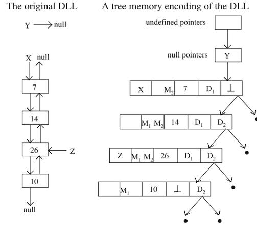
**Fig. 11** A tree memory encoding for a doubly linked list (DLL). The descriptors are mapped as follows:  $D_1 : 1.M_1$  and  $D_2 : 1.M_2$ . Only allocated nodes are present; hence the `alloc` flag is omitted
