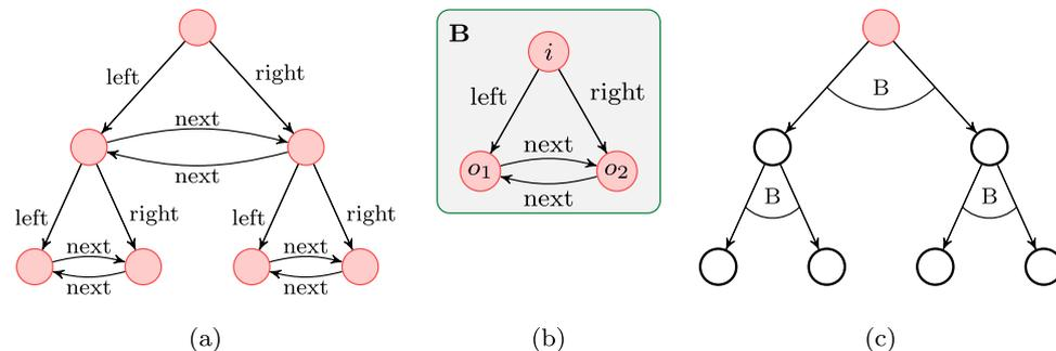
**Fig. 3** (a) A tree with linked brother nodes, (b) a pattern that repeats in the structure and that is linked in such a way that all nodes in the structure are cut-points, (c) the tree with linked brother nodes represented using hyperedges labelled by the box *B*
