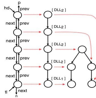
**Fig. 2.** Two spanning trees of a DLL. The middle one is an unfolding tree when labeled by  $\text{DLL}_1 \equiv hd \mapsto (n, p) \wedge hd = tl$  and  $\text{DLL}_2 \equiv \exists x. hd \mapsto (x, p) * \text{DLL}(x, hd, tl, n)$ .
