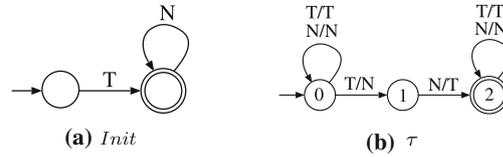
**Fig. 1** A model of a simple token passing protocol: (a) an automaton *Init* encoding the initial set of configurations  $I = L(\text{Init})$ , (b) a transducer  $\tau$  encoding the 1-step transition relation  $\varrho = \varrho_\tau$
