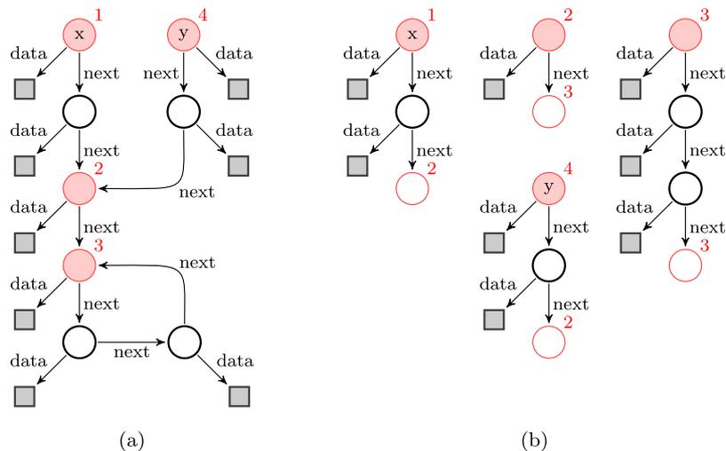
**Fig. 1** (a) A heap graph with cut-points highlighted in red, (b) the canonical tree decomposition of the heap with  $x$  ordered before  $y$
